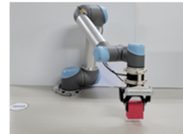
Figure 5: Block placing using a UR-5 robot.
